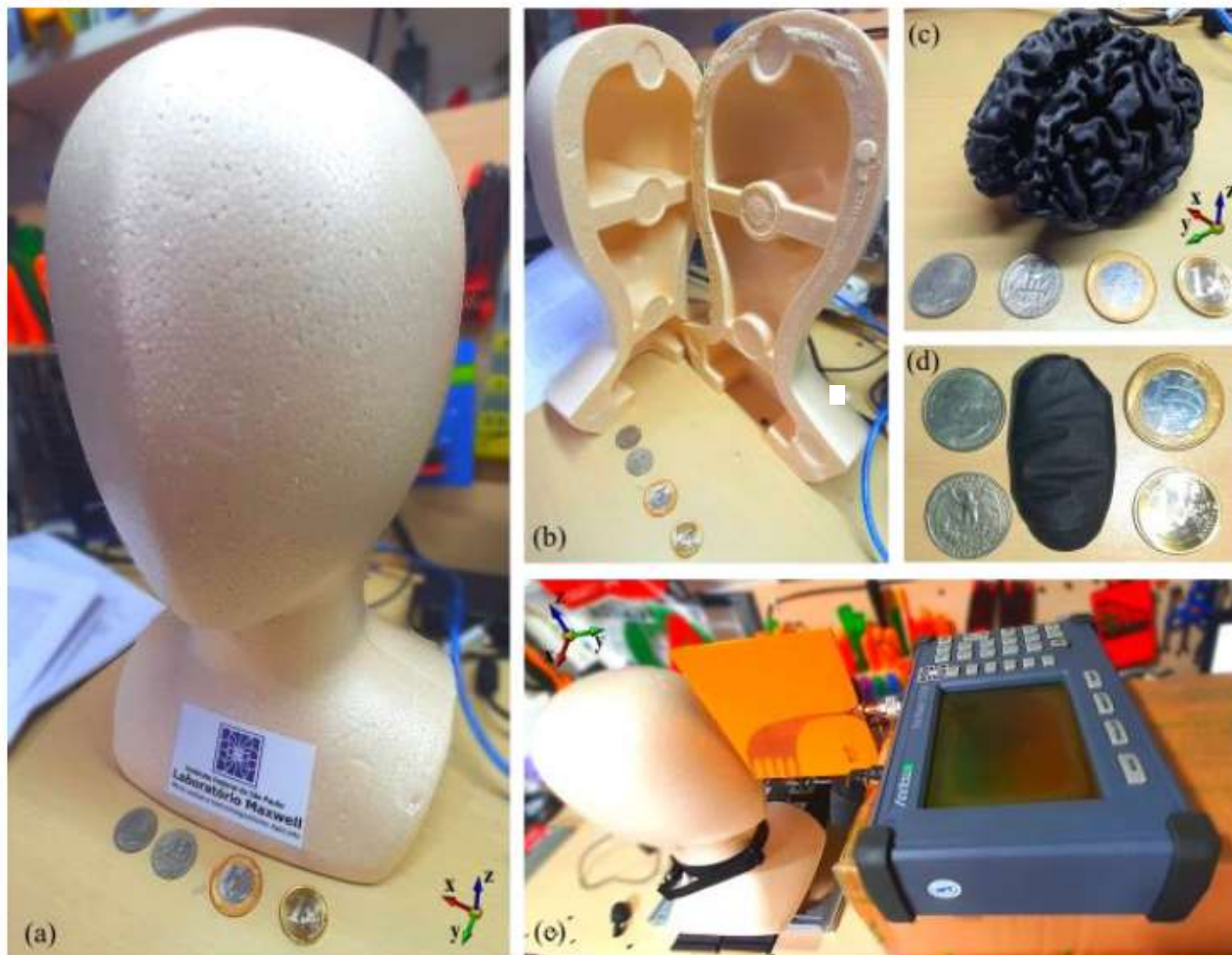
Fig. 9. A real-world scenario of the Phantom imaged by the FAVA. (a) Semi realistic and homogeneous infant Phantom. (b) Inside the Head Model, made of Expanded polystyrene (Styrofoam) from Daiso Industries CO., LTD Model YM-18-P6 C028 600 - EPS # 4, Lot # 2009BJ. (c) Infant Brain Model made with a 3D printer technique using conductive filament, composed of ABS and Graphite. (d) The Tumor Model (frontal position) was modeled with a silicone pouch, with walls of 30µm thick, filled with mineral water. (e) Proposed test setup with the Head Phantom on a mobile base controlled by the computer with steps of 1 mm; the FAVA; and the Anritsu Site Master S331B, operating with the DTF function.
